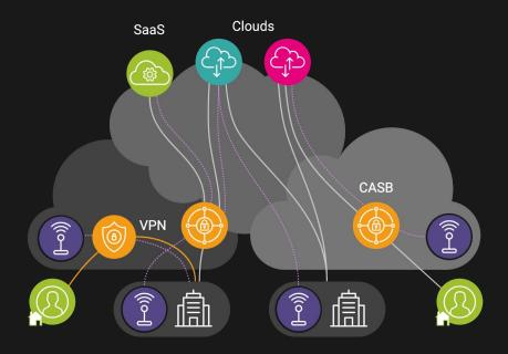
A mix of enterprise and managed Net-Tracer stations monitor network performance to data centers, clouds and SaaS applications from onsite employees and remote workers connecting via CASB and VPN gateways.
